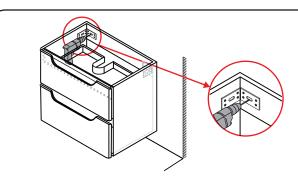
① Drill through the hole in the corner bracket on the backboard or as shown. Mark the wall according to the holes at your preferred height and drill holes in the wall.
