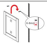
(8) Install the screws into the wall anchors, leaving enough of the screw exposed to hang the mirror - approx. 1/4"-1/2".
