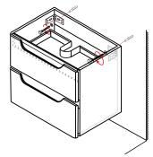
③ Fasten cabinet to wall by attaching screws through the bracket holes, and by attaching the lower brackets. Use a spirit level to ensure vanity is leveled.
