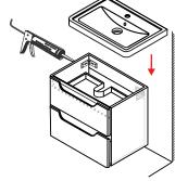
(5) Install the counter. Seal around the top of the cabinet with clear silicone sealant. Do not over apply. Allow to dry for over 24 hours for proper curing.
