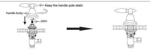
Screw the stem part (shown in picture) clockwise. Put the left handle in the same direction as the picture, keep the handle pole static, while rotating the handle body clockwise until it is firmly secured.
