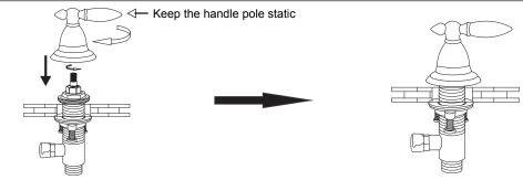
Screw the stem part (shown in picture) counterclockwise. Put the right handle in the same direction as the picture, keep the handle pole static, while rotating the handle body clockwise until firmly secured.
