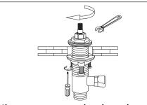
Put the screw cover back and screw clockwise until firmly secured to countertop. Then tighten the screws counterclockwise with a screwdriver.
