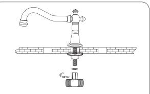
Screw the nut of the TEE joint counterclockwise, until the TEE is firmly secured.
