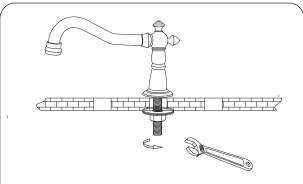
Screw the mounting nut counterclockwise, until the nut is firmly secured.
