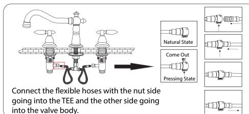
Press the quick connector button in using your fingers. Simultaneously, push in the flexible quick connect hose. Take finger off the connector button and carefully pull the flexible hose, so they snap in together.
