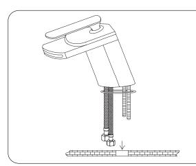
Place O-ring over water supply lines and mounting posts into the groove on the faucet base. From above, insert mounting posts and water supply lines through hole on sink.
