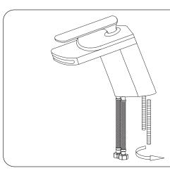
Screw two mounting posts into another two holes in the bottom of faucet body, counterclockwise.
