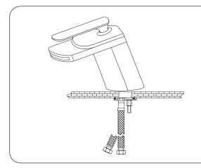
Tighten mounting nut until faucet is firmly secured to sink.
