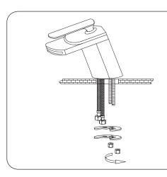
From underneath sink, secure faucet body by placing plastic washer, metal washer and mounting nut onto mounting post.
