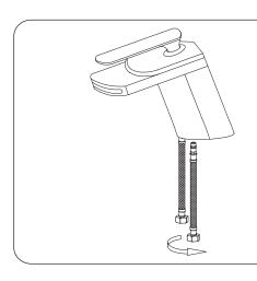
Screw two water supply lines into faucet inlet holes in the bottom of faucet body, counterclockwise.
