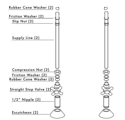
2.Once the nipple is tightened down, thread the straight stop valve onto the nipple. The handle on the valve should be facing away from the tub for easy access. On top of the valve will be a compression nut, friction
