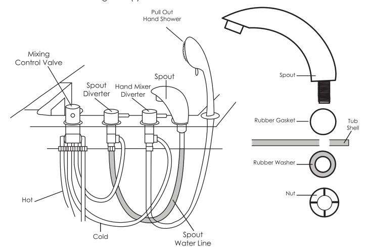
To Install the supplied spout, first place the rubber gasket on the bottom of the spout and make sure it is properly seated in its groove. Put the spout in through the hole in the tub shell (shown in the drawing above). Install the rubber washer and then the brass mounting nut. Locate the water line from the spout diverter and connect it to the threading on the bottom of the spout. Tighten all fittings and check for leaks.
