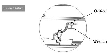
20. Replace the burner tube, then start up the oven to check oven flame, making sure it's tight and blue. Adjust the air shutter at the back of the burner tube to achieve this. Once you have the bottom pan and oven door closed, and with the broiler drawer pulled down, you will be able to see how the flame should look by viewing the flame through the broiler door area.
