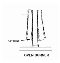
Oven burner flame can be checked as follows (without flame spreader in place):
