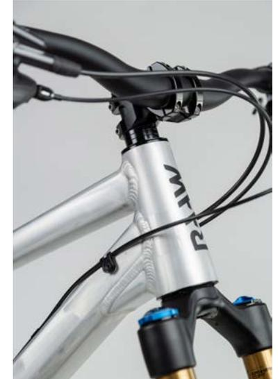
When mounting the handlebars and stem the torque settings specified by the respective manufacturer must be used. The screws must be tightened evenly and incrementally in an X-pattern.
