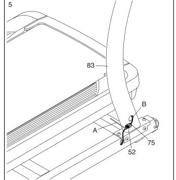
6 Set the left handrail assembly (C) on the floor in the position shown.
