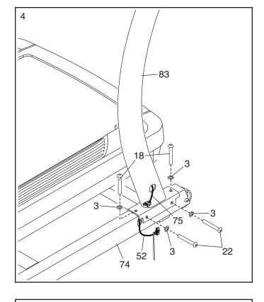
Connect the Base Wire (52) to the Upright Wire (75). The connectors should slide together easily and snap into place. If they do not, turn one connector and try again.
