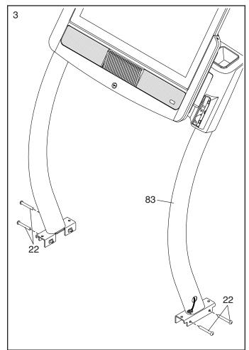
4. Set the Uprights (83) on the Base (74). Make sure that the hole with the Upright Wire (75) is on the right side.
