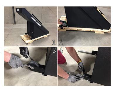
5. If you need to move the ladder, ask for assistance. Transport wheels can be reinstalled to assist in the relocation of the ladder. Roll the ladder on its transport wheels to its new location by lifting the rear end of the unit. Reminder—The ladder should never be moved with one person.
