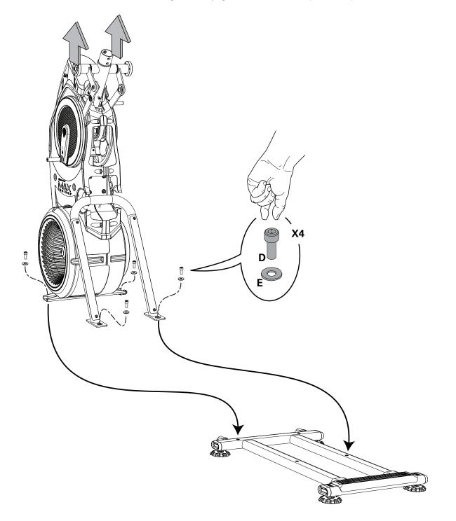
4. Attach Stabilizer Shrouds to the Frame Assembly
