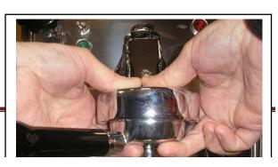
the gasket is up far enough then lock the portafilter into the group head and turn as far right as possible. Then remove the portafilter and re-install the insert basket and then work the gasket up further into the grouphead using the portafilter with the basket installed. If you are having trouble then remove the portafilter and press the screen up further by hand and then try using the portafilter again.
