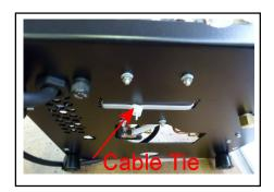
Step 2 Remove the two screws shown in the picture to the right and then pull the front panel away to expose the pump.
