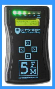
measures radiation from 40 MHz to 10 GHz and 24 GHz to 32 GHz
