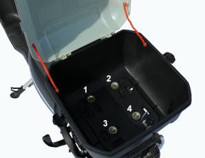
Using the keys, unlock the rear storage box and align the 4 holes in the box with the matching holes on the mounting bracket below. Secure with included hardware.
