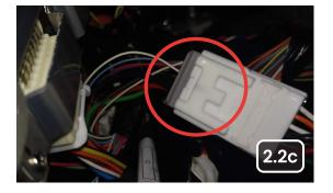
You will hear a "click" sound when the connector is properly plugged in. The centre screen will turn back on about one minute after plugging the Module into the MCU.
