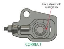
Axle Threads are lubricated with NEVER SEIZE. Stainless must be lubricated to prevent thread galling.
