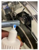
\*Use blue Loctite on threads for shock bolt only.\*
