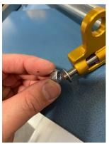
Adjustment must be done with Nylock nut. Do not force or try to over tighten during the adjustment of the belt.
