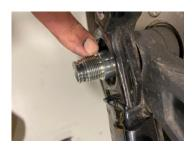
**Step 7** - Go to the right side and install the right hand side axle adjuster plate ensuring the axle adjuster key is properly mounted on the axle and not on the threads, see photo.
