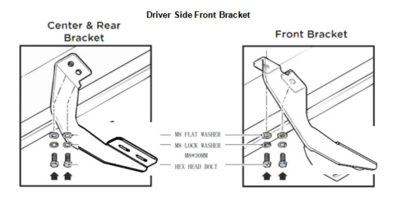
4. Repeat the above step for middle and Rear Mounting Brackets.Install three brackets on each side of the car. Install the corresponding bracket according to the serial number in the packing list.
