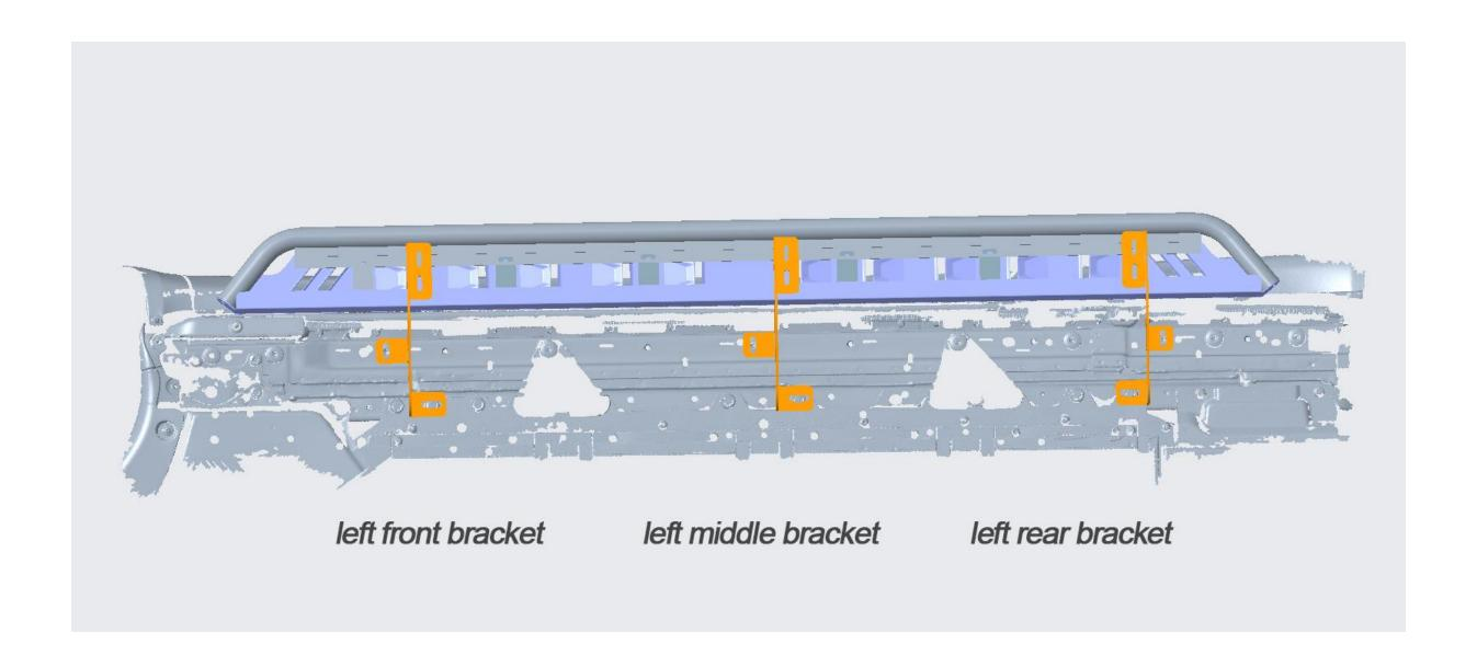
6. Install the left and right Running Boards with our M8 screws and nuts to fix them. Tighten the screws of each part, Reinstall plastic plate on the bottom complete the installation
