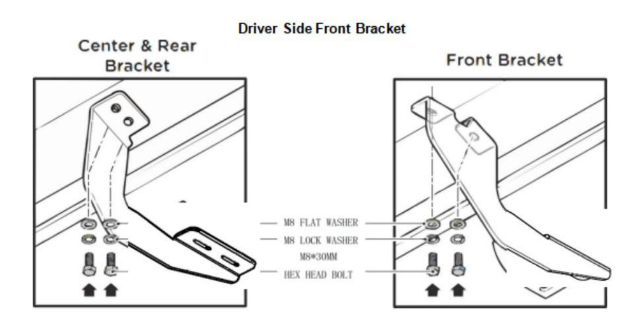
Installation diagram for Reinstall the original car screws and our screws.
