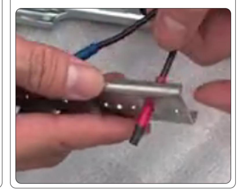
Tighten the small steel plate with six screws
