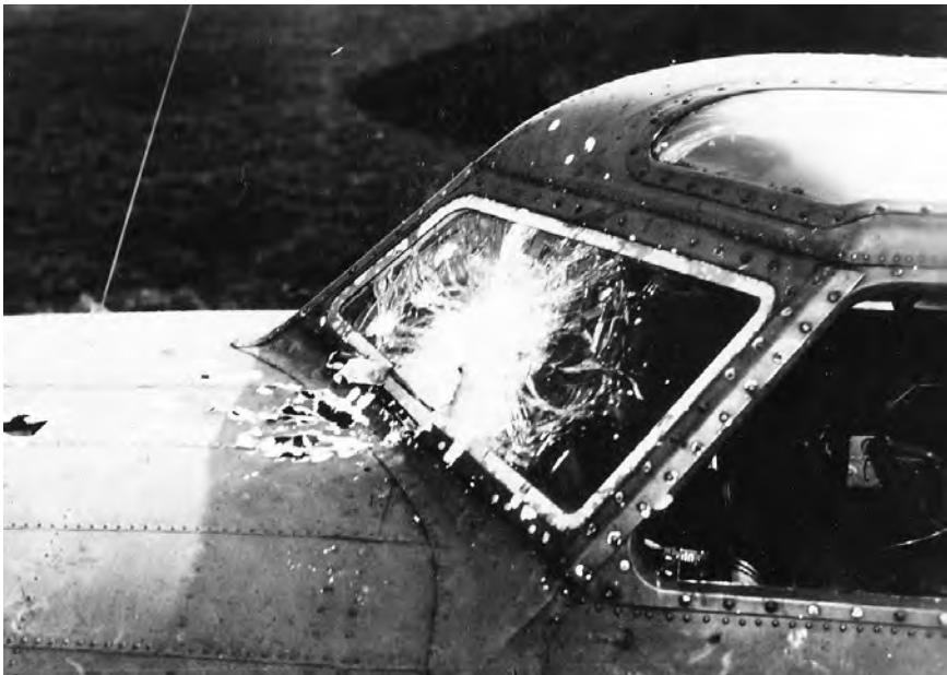
The wind-screen was severely damaged by a 20mm hit from a German fighter, which also destroyed all the instruments on the panel.
