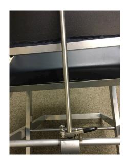
8. To adjust the headrest, release the tension release on the right side of the headrest. Manually adjust the headrest into the desired position. Once the adjustment is made secure the tension release lever back into the locked position.
