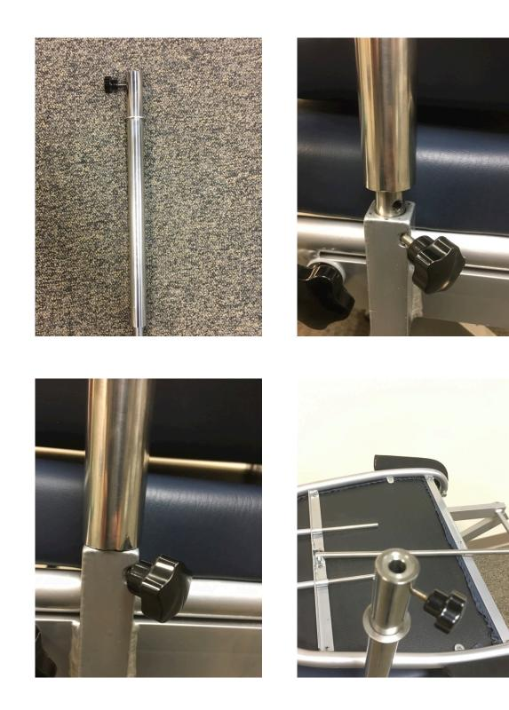
4. Install Cuspidor onto the support post.
