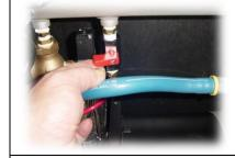
Make sure drain valve is closed.
