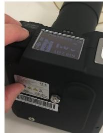
**Diagnosis:** The good news is there is nothing "wrong" with your machine! The MaxRay has a safety feature that will freeze the machine if the exposure button is pressed too long (past exposure) or too soon (before "READY") or if both the buttons are depressed simultaneously. This feature protects the machine from continuously firing radiation if a button was to get stuck or inadvertently triggered.
