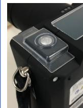
**NOTE:** We developed a silicon cap to mitigate issues with disinfectant, liquid and dirt penetrating the button and damaging the main control / power board.
