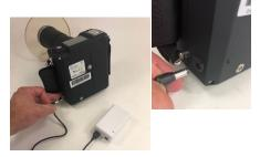
Prescription: To "reset" the machine find your external back-up battery and plug it into the back up battery port below the handle on lower lefthand side of the machine. Count to 5 and unplug the back-up battery. This flips the power supply from the internal battery to the external battery and back to the internal battery, thus resetting the machine. (note the external battery must be charged for this procedure to work).
