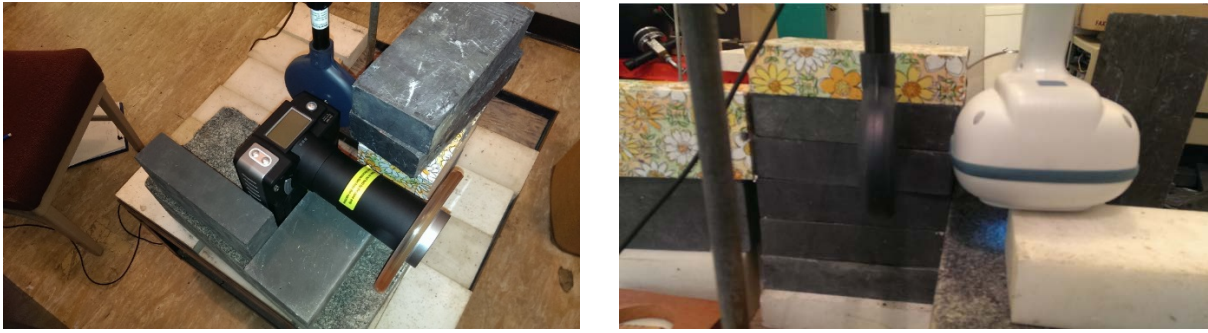
Figure 4. Experimental arrangement for leakage measurements
