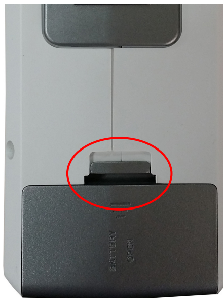
Figure 7.10 Battery cover separation
