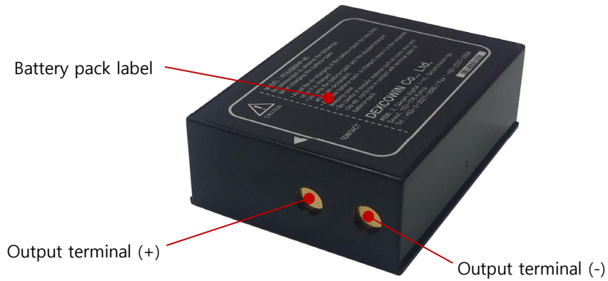
Figure 6.8 Battery pack parts
