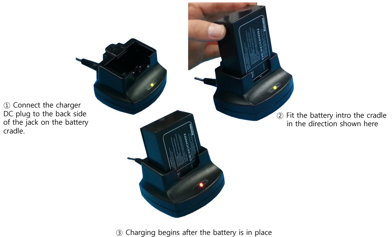
Figure 7.15 Connecting the battery into the cradle
