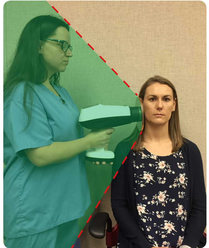
The backscatter shield provides a safety zone to the left of the green line.
