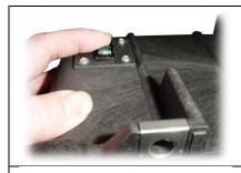
Turn the vacuum power switch on when needed.
