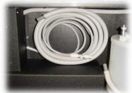
Disconnect saliva ejector line and pack into case.
