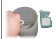
Mix non-foaming vacuum system cleaning solution and run solution through HVE valve.
