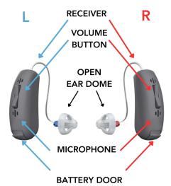
NOTE: Battery door is on/off switch
