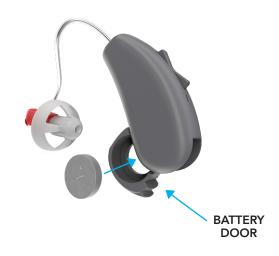
Remove tab on new battery to activate. Open door, insert a fresh 312 battery with the positive '+' side facing up and close the door to turn on the hearing aid.
