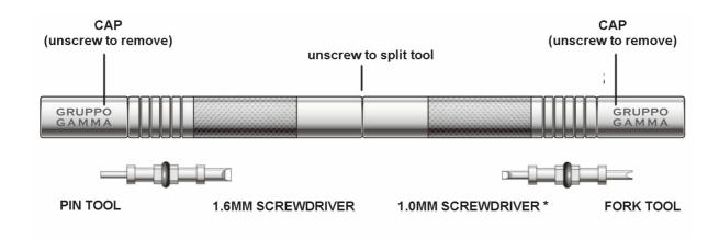
\* Earlier versions are fitted with 1.6mm screwdriver instead, for use with Mk I Nexus models
