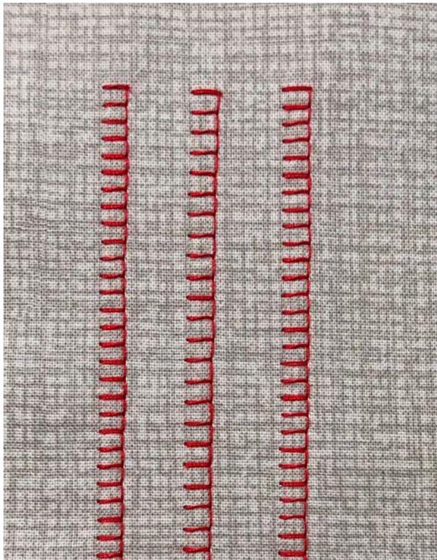
Row 1 Row 2 Row 3 Programmed settings 4 mm width 3 mm length 4 mm width Default length
