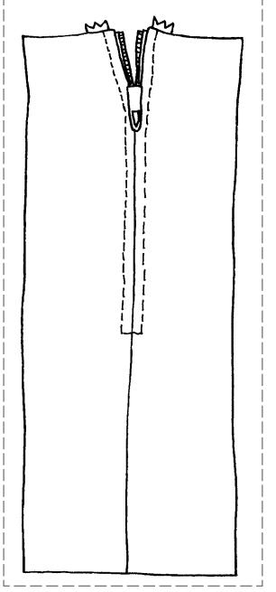
Note: The invisible zipper can be used in place of a conventional zipper when an uninterrupted design line is desired.
