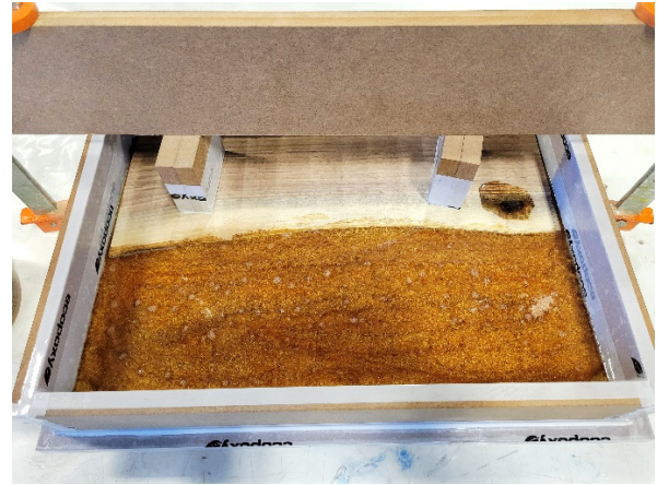
Figure 19: Resin poured up to top edge of slab
