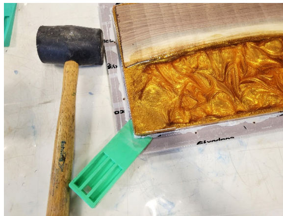
Figure 22: Demolding in progress
