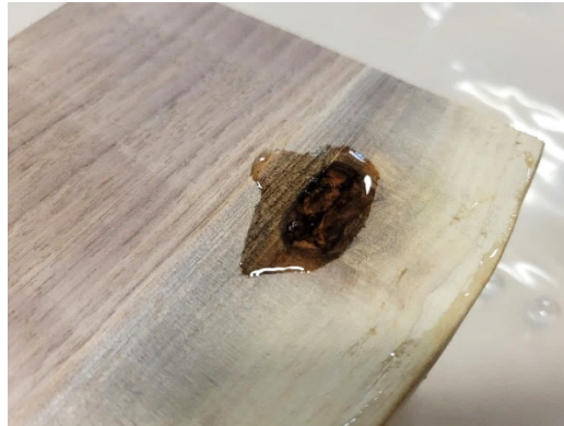
Figure 7: Knot in wood covered with FlowCast SPR
