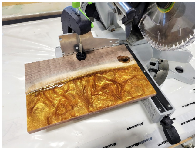
Figure 23: Edges cut with a miter saw
