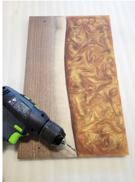
Figure 28: Clearance holes for serving tray bolts
