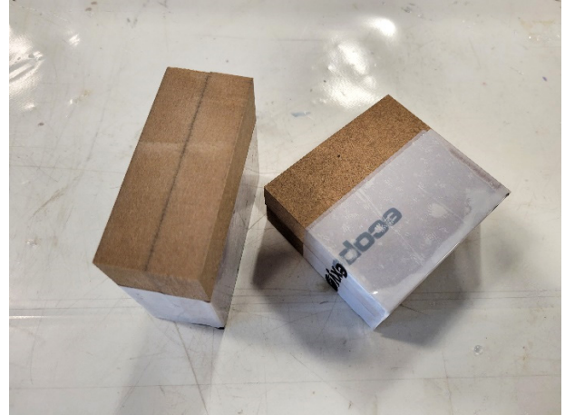
Figure 10: MDF blocks taped together for clamping
