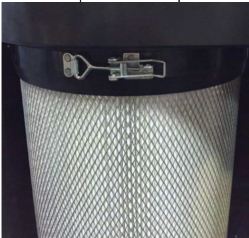
Figure 8: Hold canister from bottom when releasing clamp
