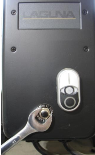
Fig. 2C: Replacing Overload Protector
