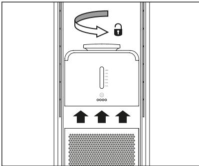
1. Lift the cover with the attached filter carefully. The cover attaches magnetically to the main body.
