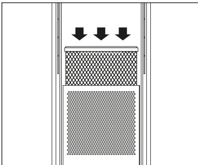
3. Unpack the new filter and attach it to the cover (snaps in, no screwing)
