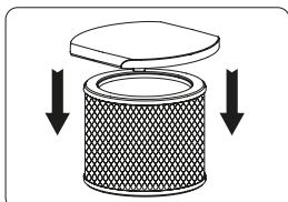
Insert HEPA14 Filter unit into the cover.
