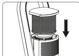
Apply the cover with the attached filter and lock to main body.
