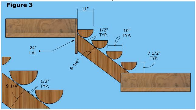
Now that you have the lengths and angles cut the stringer, don't forget to notch the bottom around the floor or landing. Attach the top with lags through the 24" LVL. Attach the bottom with lags through the floor. There are two different sized brackets, the shorter brackets are for the bottom tread. Starting at the top, take a bracket set a tread in the bracket and level the tread. Measure down 7 1/2" mark the placement of the bracket and lag into place. See figure 4.
