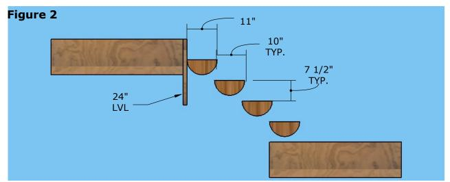
Mark a Line 1/2" below the bottom of the stair treads. **THIS WILL BE THE HEIGHT OF THE BRACKETS.** This is the top of the stringer, measure down 9 1/4". Mark a line for the bottom of the stringer. Now you have the length and angle to cut the stringer. See figure 3. It is very important to notch the bottom of the stringer around the floor system. This is what will hold the stair in place.
