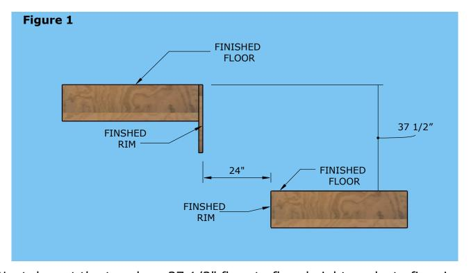
Next, layout the treads, a 37 1/2" floor to floor height works to five rises at 7 1/2", measure down 7 1/2" from the finished floor and make a level line. The treads are 11" so your run will be 10". Measure out 11" and make a plumb line. Take a tread and put it even on the level line and up against the rim and mark. See figure 2, measure down 7 1/2" from the top tread and mark a level line. Measure out 10" from face of the first tread and plumb a line. Repeat until all treads are marked.
