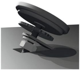
The thermometer for the pizza oven is mounted with the various parts as shown in the image above.
