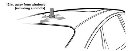
NOTE: For aluminum roofs, an **adhesive disk** is included to mount the outside antenna (do not use if outside antenna will magnetize to the top of your vehicle).
