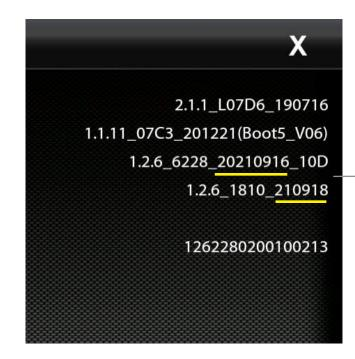
2. Note the APP and System Versions and head over to the UN1810 product page on stingerelectronics.com. Select the New Firmware Tab on the product page. The most current firmware will be listed with a date. The 8 digits of the APP Version is the APP Version date code (YYYYMMDD). The 6 digits of the System Version is the version date (YYMMDD). If the date code of either the APP or System firmware is older than the current firmware on the website, proceed to Updating System Firmware.
