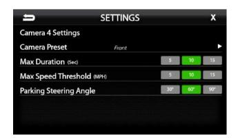
The settings shown above will activate a Front camera, when shifted into Drive, for 10 seconds or when vehicle speed reaches 10mph. If Park Assist is active, the Front camera will activate whenever steering wheel rotation is 60° or more.
