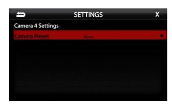
From the individual Camera Settings page, Camera Presets can be assigned and trigger parameters can be edited.
