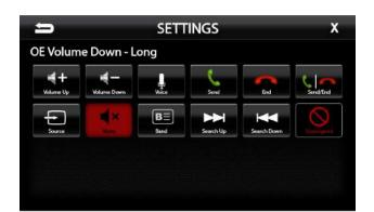
Select any of the functions shown to assign that function to the button.
