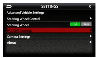
To view or change the default steering wheel control functions, select **Advanced Vehicle Settings > PAC SWC Settings** from the Installer Settings.
