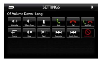
After pressing a button assignment, a menu of functions will be displayed, with the current function highlighted.
