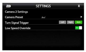
The settings shown above will activate the Bed Camera for as long as the turn signal is active and vehicle speed is over 3 MPH.
