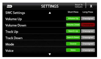
The default settings will be displayed. To change or add a SWC function, touch the corresponding Short or Long Press button assignment.
