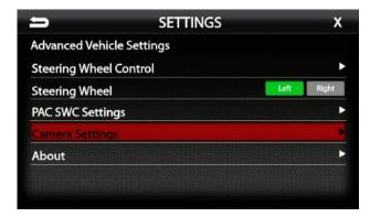
To view or change the camera settings, select **Advanced Vehicle Settings > Camera Settings** from the Installer Settings.
