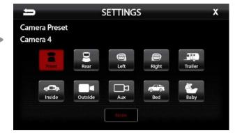
Selecting Front will activate and label Camera 4 as the Front camera. Use the Back arrow to edit any available trigger options.
