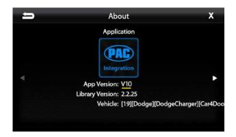
3. Note the App Version and head over to the UN1810 product page on stingerelectronics.com. Select the Firmware Tab on the product page. The last digit of the App Version is the revision. If the revision number of the installed PAC Integration APK is older (smaller number) than the current revision on the website, proceed to Updating the PAC Integration APK.
