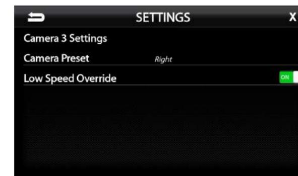
The settings shown above will activate the Right Camera for as long as the turn signal is active and vehicle speed is over 3 MPH.
