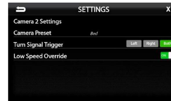
The settings shown above will activate the Bed Camera for as long as the turn signal is active and vehicle speed is over 3 MPH.
