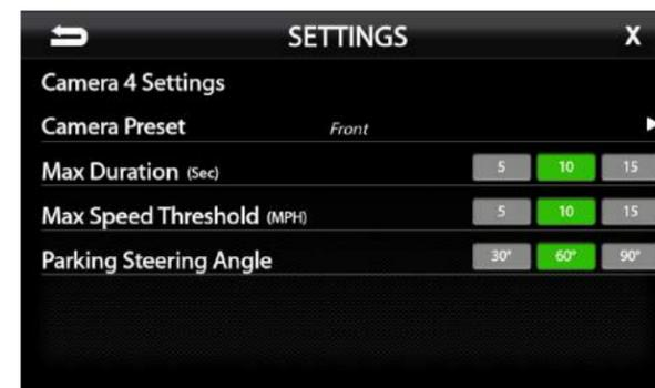
The settings shown above will activate a Front camera, when shifted into Drive, for 10 seconds or when vehicle speed reaches 10mph. If Park Assist is active, the Front camera will activate whenever steering wheel rotation is 60° or more.
