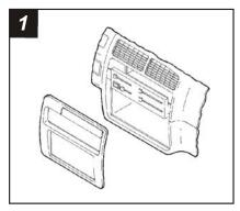
Disconnect the negative battery terminal to prevent an accidental short circuit. Pull the cupholder out. Unclip the radio trim bezel and remove. Remove (4) screws securing the factory head unit and disconnect the wiring.
