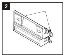
Cut and remove the middle mounting legs on the *Radio Housing*. Skip to the Installation Instructions for ALL VEHICLES on Page #3.
