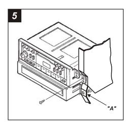
Re-connect the battery terminal and test the unit for proper operation. Mount the head unit/kit assembly to the sub-dash with (4) screws previously removed in step #1. (For the Standard Cab Pickup 1992-95, slide the lower mounting tabs behind the dash bracket and secure from behind ("A"). (see Fig. A)
