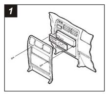
Disconnect the negative battery terminal to prevent an accidental short circuit. Open the center armrest door. Unclip the parking brake trim panel. Unclip the gear shifter trim panel and remove the panel. Remove the climate control knobs. Remove the climate control trim plate and (2) Phillips screws exposed. Unclip the dash trim bezel and remove. Remove (4) Phillips screws securing the factory head unit and disconnect the wiring.
