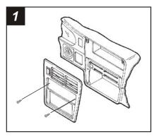
Disconnect the negative battery terminal to prevent an accidental short circuit. Remove the climate control knobs. Unclip the climate control trim panel and remove (2) Phillips screws exposed. Unclip the dash trim bezel, lift up on the bezel and remove.
