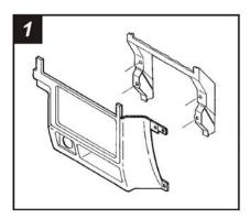
Disconnect the negative battery terminal to prevent an accidental short circuit. Remove (3) screws and (1) 10mm bolt from the driver's side speaker panel and remove the panel. Remove (1) 10mm bolt from the bottom of the passenger's side speaker panel. Remove (3) screws from the side of the panel and remove the glove box. Remove (4) screws securing the factory head unit and disconnect the wiring.
