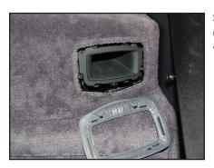
**STEP 3**Carefully unclip the trim around each of the enclosure ports as shown.
