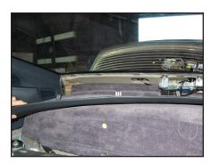
**STEP 9**Carefully unclip the rear trim panel as shown.
