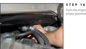
From the engine bay, insert the assembly up through the empty grommet hole.
