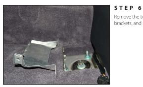
Remove the two small carpeted panels, unbolt the enclosure brackets, and remove the brackets from the vehicle.
