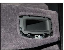
**STEP 4**Remove the bolt under each of the enclosure ports.
