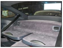
**STEP 2**Fold down the rear seats to gain access to the factory subwoofer enclosure.
