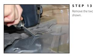
Remove the two grommets near the back of the vehicle as
