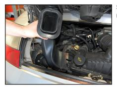
**STEP 14**From the engine bay, remove the air intake tube as shown.
