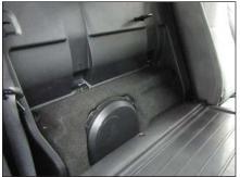
Connect the speaker cable to the terminal cup on the side of the enclosure, and place the Stealthbox® into position, as shown.
