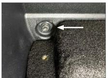
Remove the factory bolt from the back of the storage pocket on each side of the enclosure. These will not be reinstalled.
