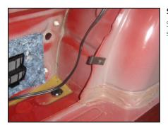
STEP 9 Slide a U-Nut over the factory hole in the wheel well as shown.
