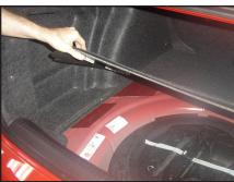
STEP 4 Remove the trunk floor panel.
