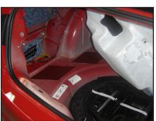
STEP 7 Pull the trunk liner away from the side of the trunk as shown.
