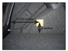
**S T E P 2** Place the supplied wax square onto the driver's side rear cargo panel.
