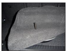
Thread the supplied socket cup screw into the rear of the Stealthbox®.
