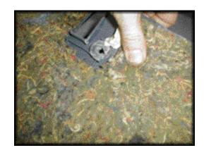
STEP 5: Reinstall the lower rear trimpanel. Install the supplied bracket onto the Stealthbox. Place the Stealthbox in the vehicle and drill the two holes through the plastic panel using the holes in the bracket as guides. The holes should align with the holes in the spacers installed in Step 4.
