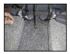
STEP 10: Drill through factory threaed hole using 1/2" drill bit.
