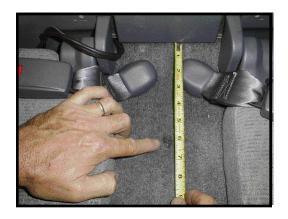
STEP 8: Cut carpet around factory bolt (Approximately one inch diameter) so that the bolt could be easily removed.
