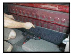
STEP 3: Insert supplied speed clips onto the bracket located on the lower area of the rear wall of the truck. The two clips go over the inner two holes on this bracket.
