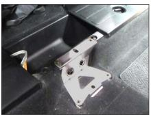
**STEP 4** Remove the two bolts from the console bracket.
