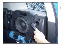
**STEP 6**Remove the upper right mounting bolt.
