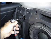
**STEP 5**Remove the upper left mounting bolt.
