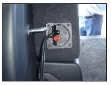
**STEP 13**Run speaker wire from the amplifier location to the Stealthbox®. Double check the woofer for proper operation.
