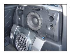
**STEP 4**Loosen the four exposed screws and remove the grille panel.
