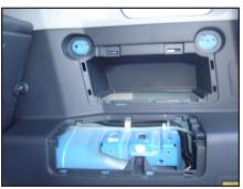
Remove the factory "woofer" system or the pocket from the vehicle.
