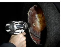
Using a 1/2" drill bit through the existing hole in the Stealthbox®, mark the plastic side panel. Do not drill through the panel at this time.
