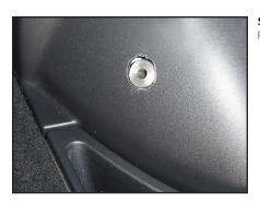
**STEP 12**Place the Spacer into the hole drilled in the side panel.
