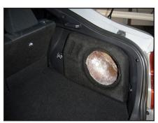
**S T E P 2**Remove the woofer from the Stealthbox®, and place the enclosure into position as shown.
